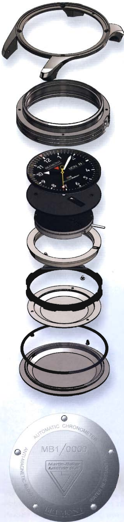
The movement is encased in a faraday cage, which is surrounded by shock-dampening movement suspension and then sealed behind a screw-down caseback.
